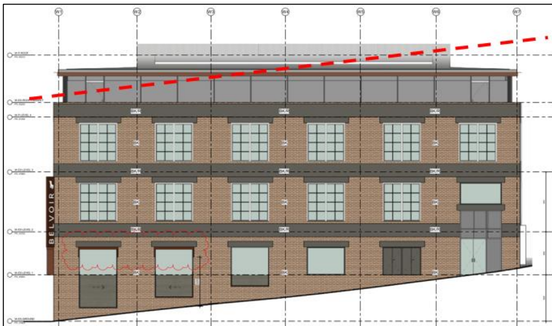
Figure 23: Southern (Belvoir St) elevation showing the 15m height control dashed
